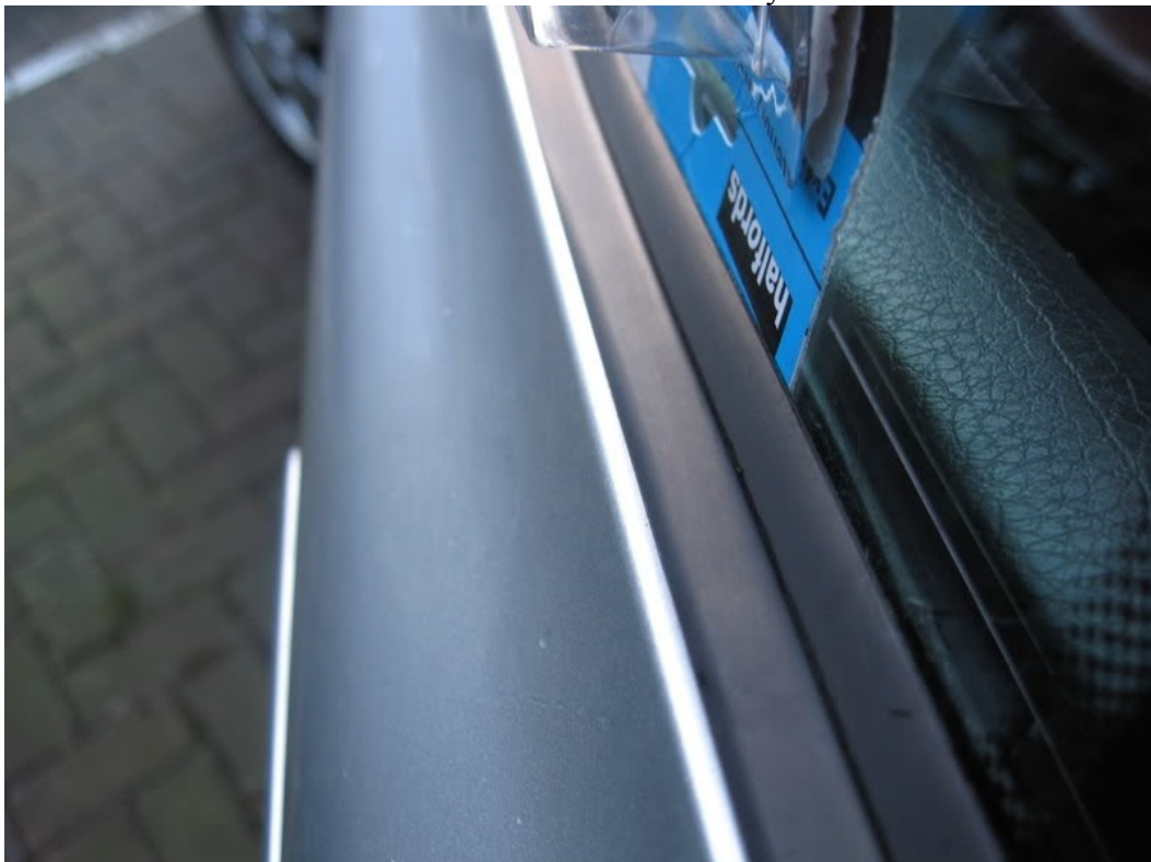
Cardboard space between old seal and glass.
