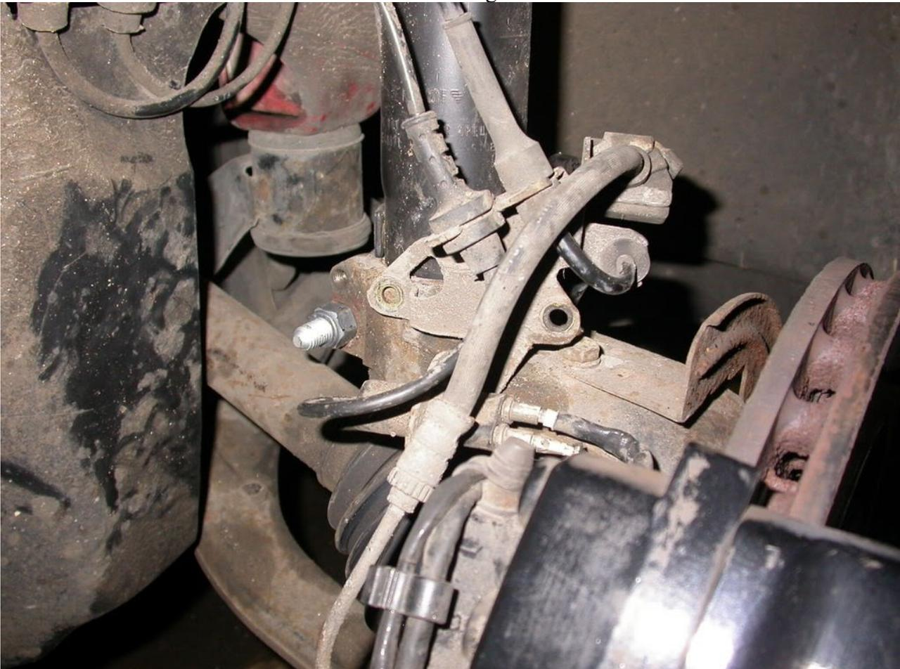
5. Remove the 2 (10mm) bolts holding the clips for the brake hoses and pad wear sensors – this is just to help improve access and allow you to remove/refit the parts
