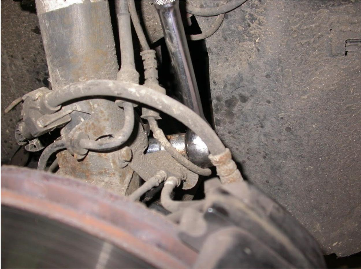
6. Remove the locking nut on the pivot clamp bolt (16mm) and remove the bolt.
