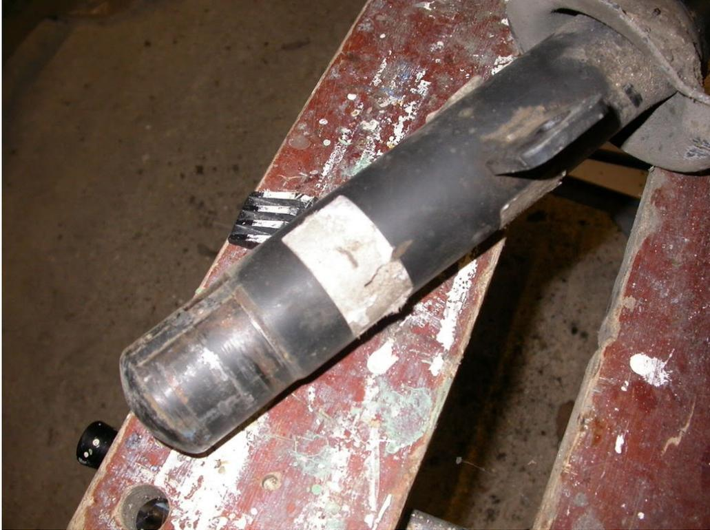
20. Fit the strut components f, e, and d to the new strut, and insert into the spring.
