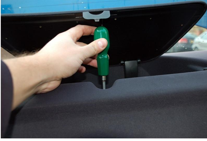
4. Lift the rear parcel shelf up and out and put to one side. There are some stick on bits of foam at the back which can start to come off and make it feel like some thing is caught. don't worry, just pull a bit harder and retrieve the foam if it pulls free.
