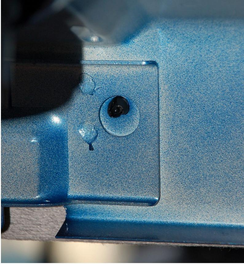
They can be released by pushing a flat head screw driver in the back so the centre piece comes out
