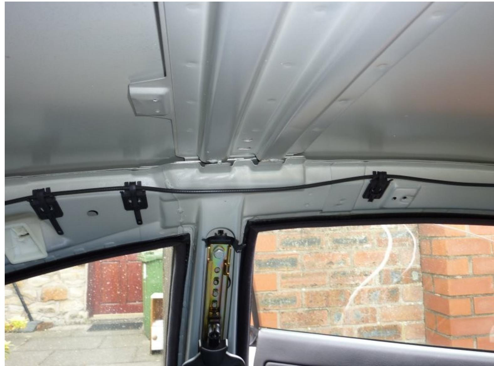
The rear covers do not need to be completely removed, just pulled away starting at the top and working down.
