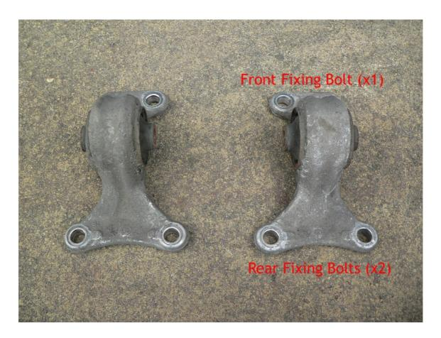
You can see in this image which side they are from. Of the two forward bolt holes, only the one nearest the outer edge of the car is used (the one nearest the sill). My old ones are labelled Kleber on the rubber - the new ones are Michelin (the Peugeot part no. for item 16 has changed since the image above, possibly to reflect the use of Michelin rubber).
