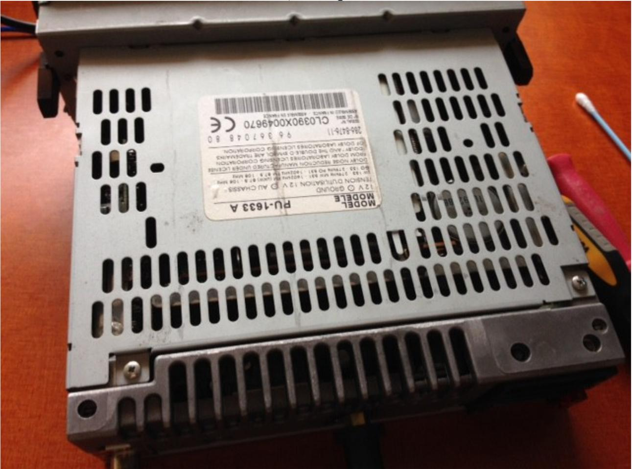
Firstly, remove the headunit from the dash, unscrew the 2 screws that are on the top of the unit and take off the lid.
