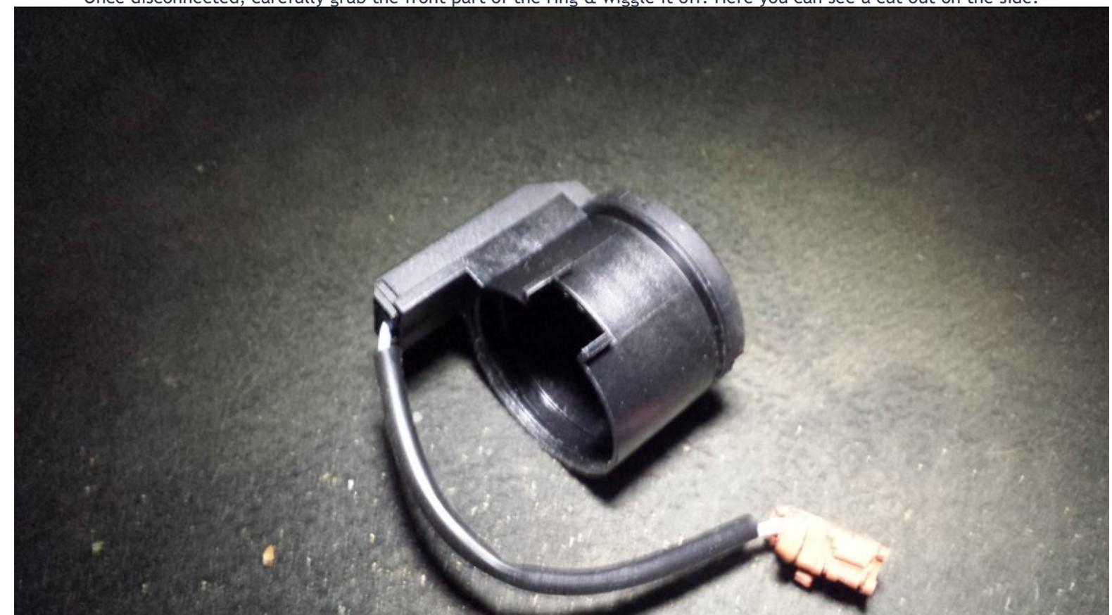
Fitting is easy too. With the cut out above towards the dash, it slips over the metal part of the barrel, the black chunky part of the new aerial points almost downwards:
