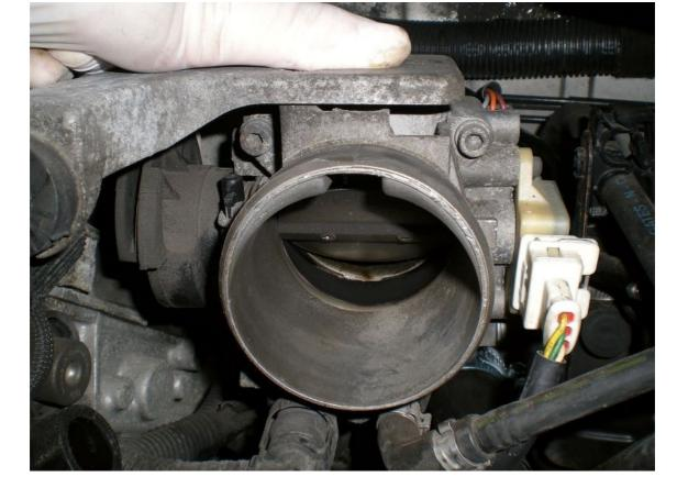
10. Refitting is not quite the opposite of removal. Put the pipes on the ICV with some jubilee clips just tight enough so they don't slide around. Fix the short L-shaped pipe to the inlet manifold and screw the clip back into the throttle. Arrange the jubilee clips so you can get a screwdriver to them. Put the airbox side back together first and then finally tighten all the
