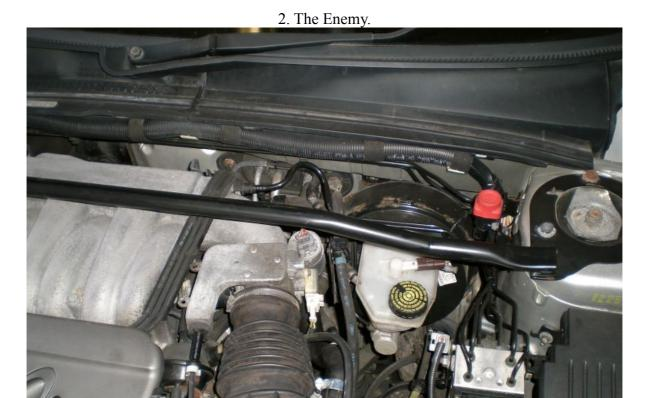
3. Unplug the electrical connector from the ICV (push the metal bar in and pull the plug) and remove the 2 allen screws to the side of it holding the clip to the throttle body
