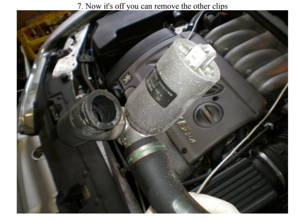
8. This is nearly £200!!!! Blast it with carb cleaner until it's clean. If you give it a GENTLE (£200 gentle!) twisting motion, you should feel the valve opening and closing smoothly. If it feels gritty, get back at it with the carb cleaner. I'd do the pipes you removed too.
