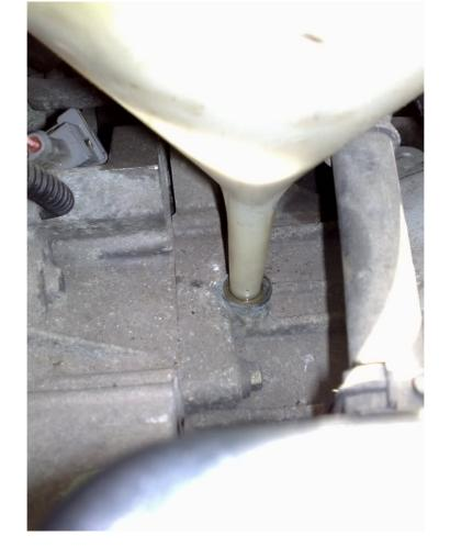
There is a slight lip around the hole which this sat into, helping me to hold it steady while the funnel was filled
