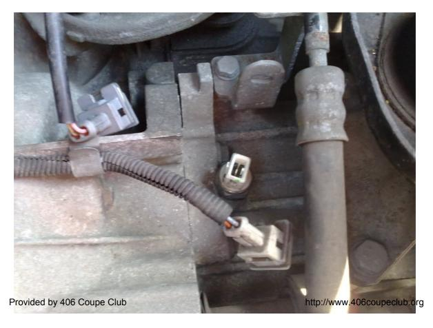
Once off, you will need a deep-reach socket, or correctly sized spanner to undo the sensor. This is the easiest way of refilling the gearbox with oil when it comes to it.
