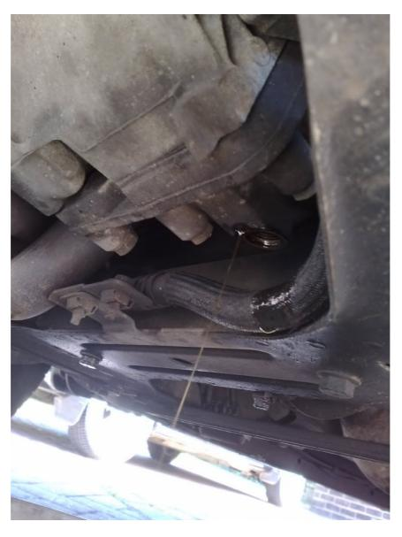
Due to the gearbox only holding two litres, and the reverse light sensor being removed, it will not take long for most of the oil to drain out and leave a dribble....
