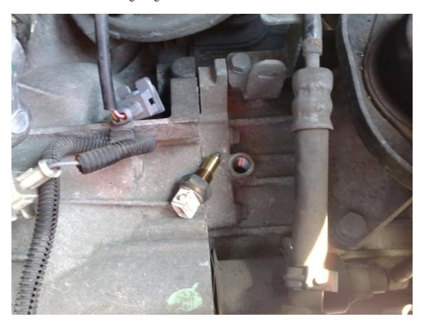
Now that you have somewhere to fill the gearbox up, it would be a good idea to empty it!! lol Locate the gearbox sump nut. The nut is located at the rear of the gearbox. From underneath it looks like this:
