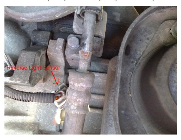
The wires come off this sensor with ease, though in my case it was easier for me to unclip the metal securing pin rather than push it in to remove it.
