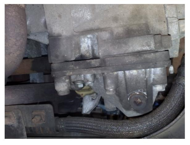
Using a sump-put-key (same size as the one for the engine oil), crack off the sump-nut for the gearbox but do not remove.
