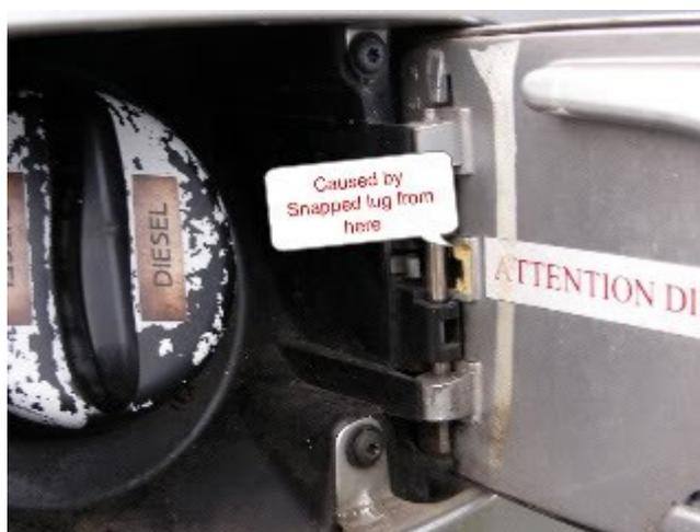
The solution is simply a piece of sprung steal.
