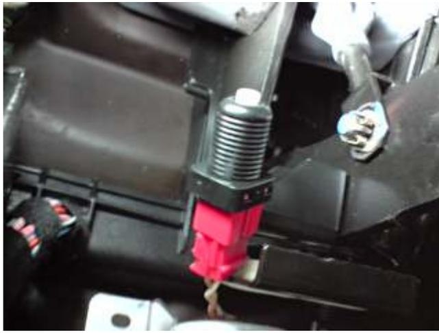
Make sure the key is removed from ignition (just in case) and detach the sensor
