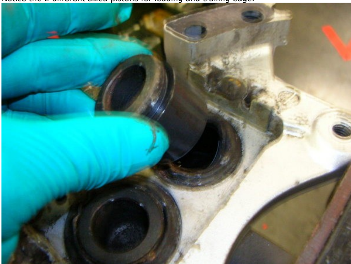
The rubber seals can then be removed using a small flat blade screwdriver (i used a watchmakers) pull up on the seal whilst levering it out of the recess.
