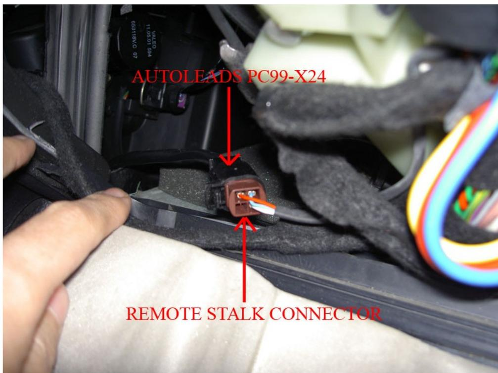
Connect together all the parts of the PC99-X24, and you'll see the Headunit-end of the unit is simply an ISO male to female. So you'd think you could plug one end into the car, and the other end into your Headunit. But when you do this, you won't get any sound !
