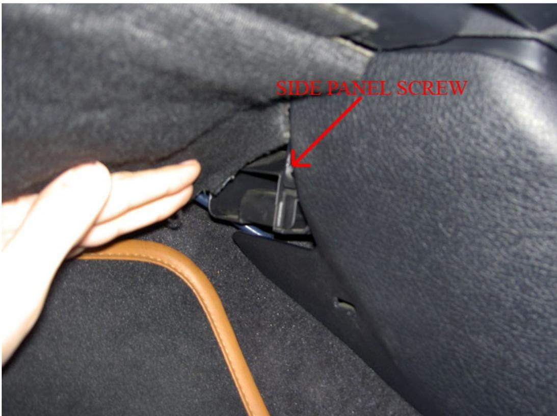
The other screws are under the ashtray. Open the lid, and pull the whole assembly out. Carefully disconnect the bulb holder, and unclip the gear gator so you can move it out of the way. Take out the two side panel screws.
