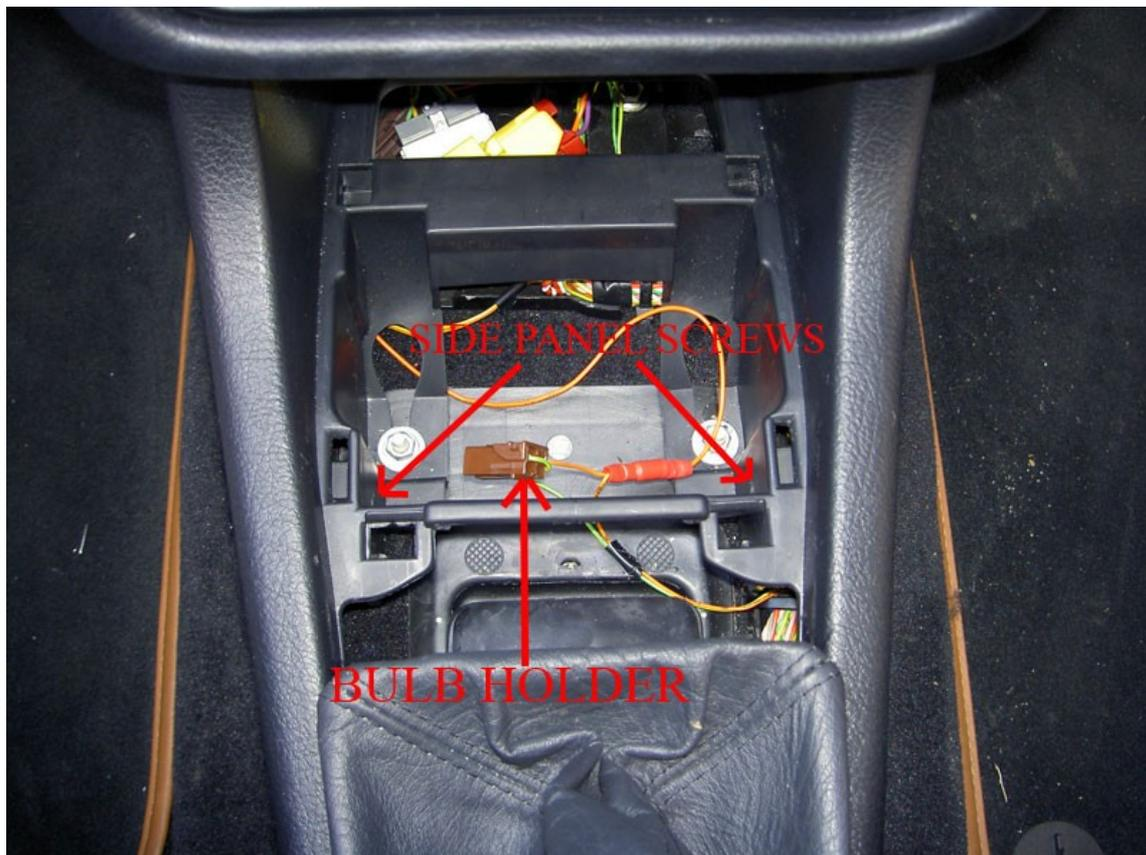
Now you can remove the two side panels. They just unclip, and need to be wiggled free. Once the panels have been removed, you need to remove the airduct pipes – again, they just unclip and pull off.
